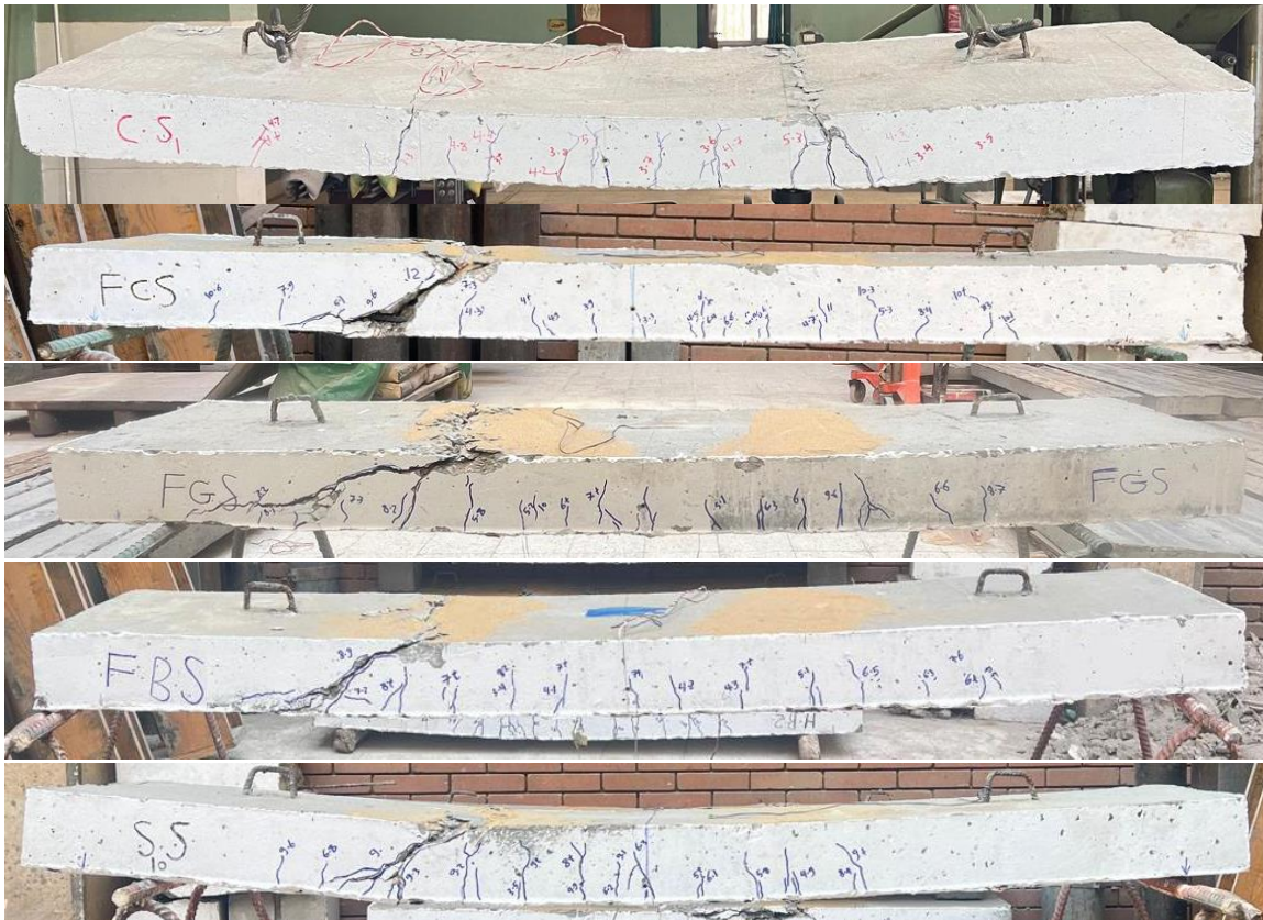
Figure 5: Cracks pattern of slabs tested under static loading
