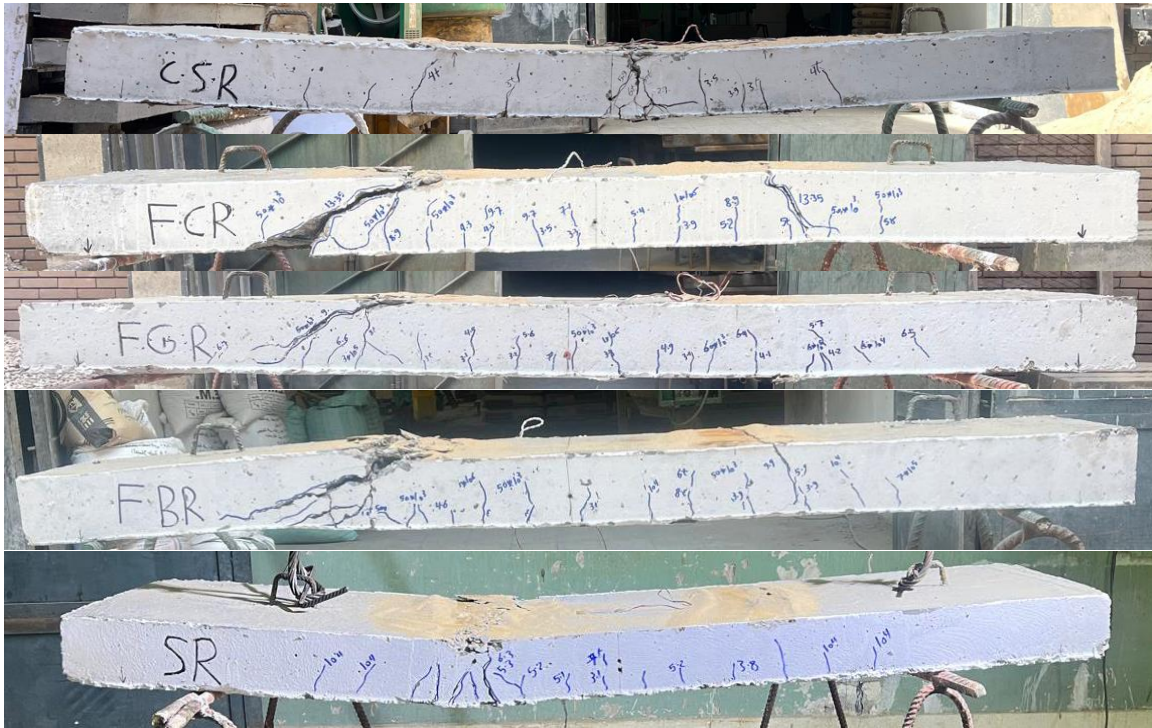
Figure 6: Cracks pattern of slabs tested under repeated loading.
